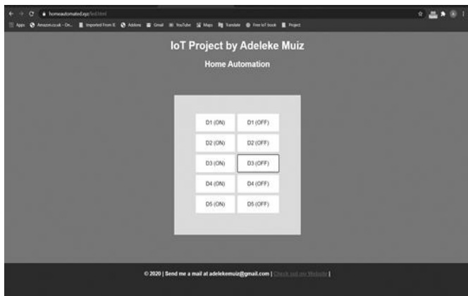
Fig. 9 User interface created for appliance control using HTTP protocol
