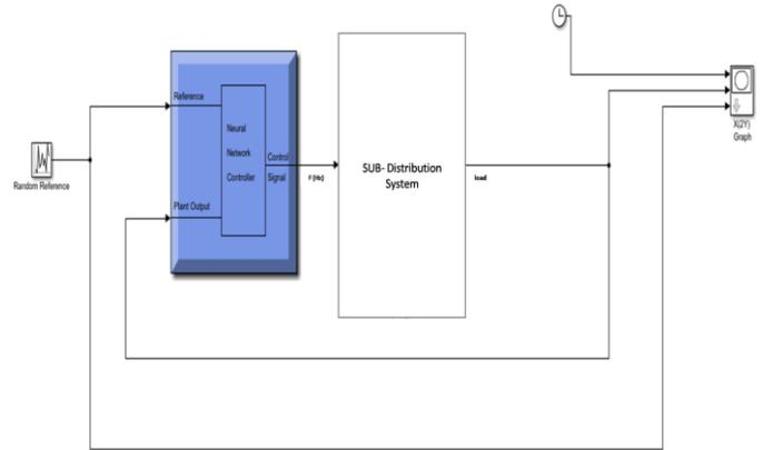
Figure 5: Simulink model of the neuro frequency controller
