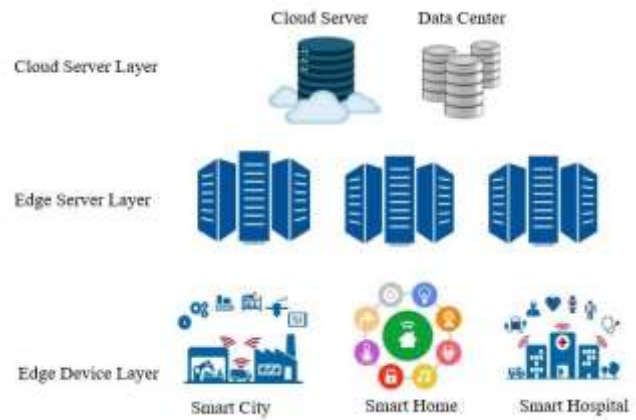
Fig. 2. Three-layer architecture of MEC edge devices through different wireless interfaces.
