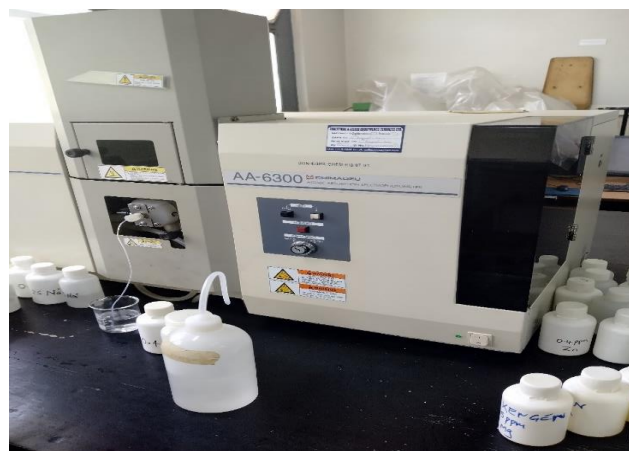
Figure 2.5: A photo showing the process of water injection into the machine to zero the reading.
