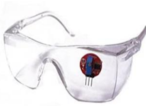
Fig. 6. Infrared Eye Blink Sensor Module.
