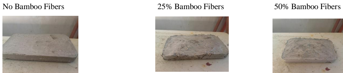
Figure 1. The Different Concrete Cement Used in the Experiment.
