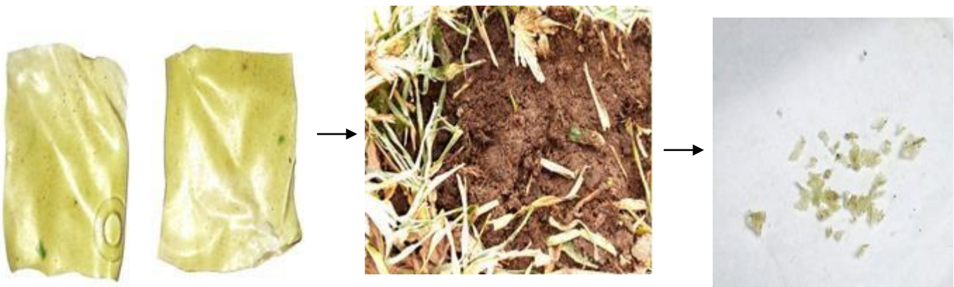
(a) Nylon before Soil Burial Test (b) Biodegradable nylon buried in the soil (c) Nylon film after one Week
