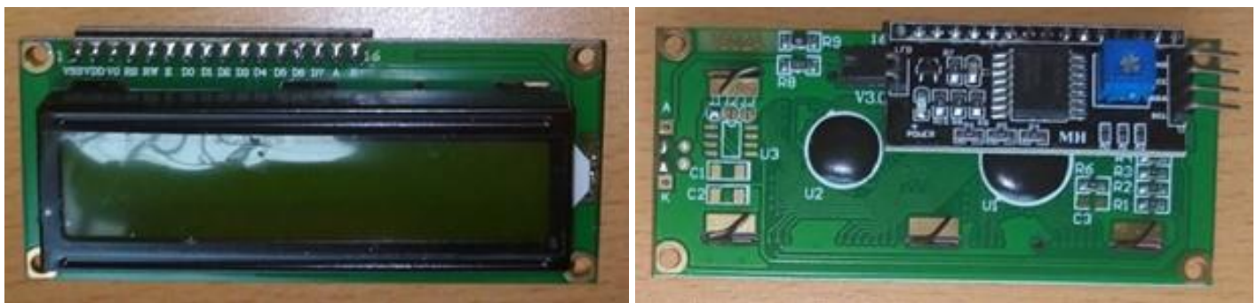
Fig. 4.4: 16x2 I2C LCD
