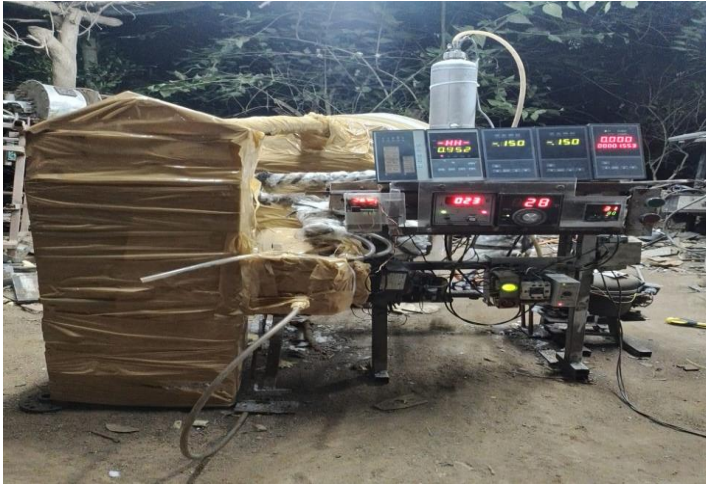
Figure 3. Fabricated Vapor recompression system
