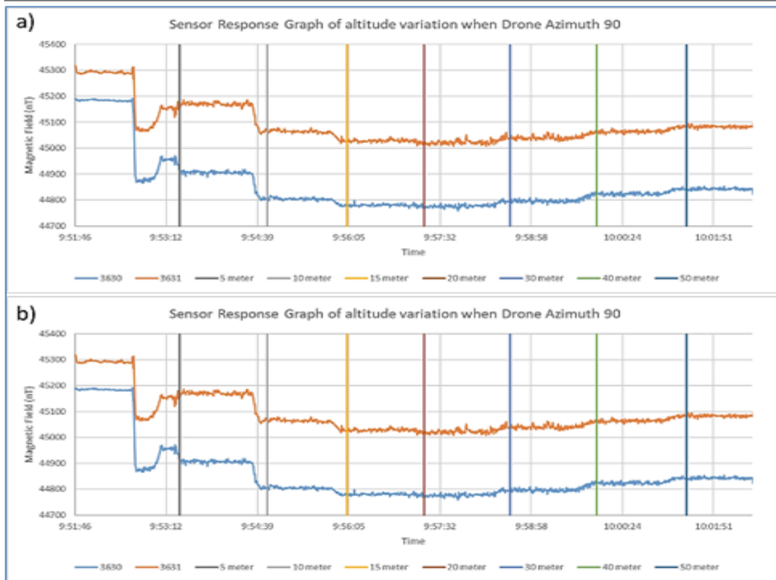
Fig. 3 Altitude variation testing with drone face azimuth (a) 90° East and (b) 0° North.
