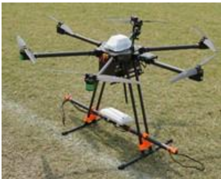
Fig. 1 Configuration of the drone magnetometer
