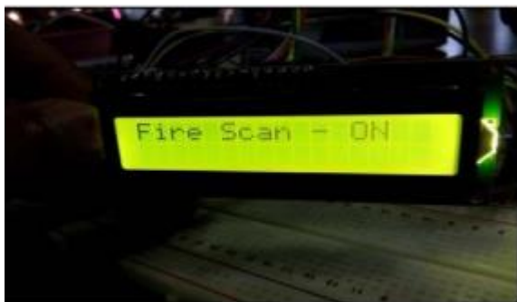
Figure 4.9. When the fire is still not detected, LM35 is in ready mode.
