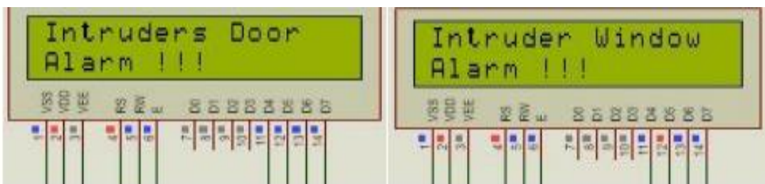
Figure. 4.7a and Figure 4.7b Output from the display when at least one switch in the PIR sensor group is activated
