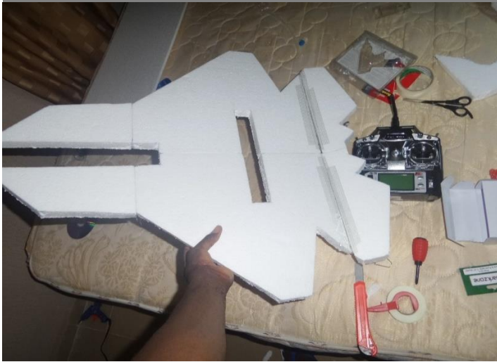
Plate 6: Nose, wing and elevons assembly
