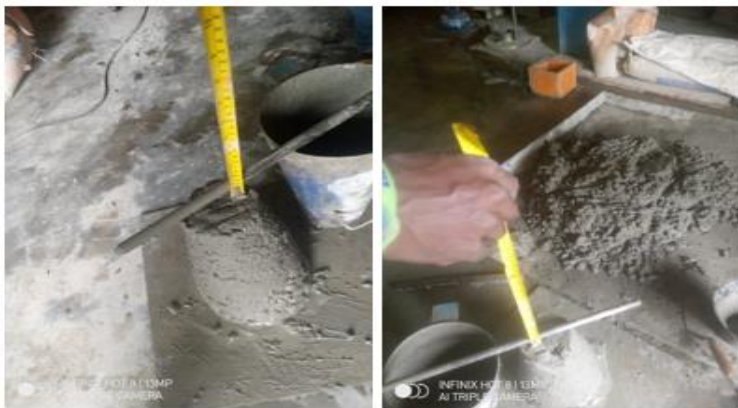
Fig. 2: Workability of concrete (Slump Test)
