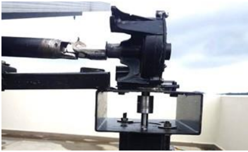
Fig 3: NEMA 23 stepper motor coupled with the shaft
