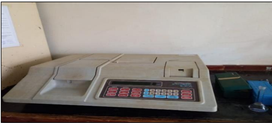
Figure 4: UV-VIS Spectronic spectrophotometer for phosphate determination.
