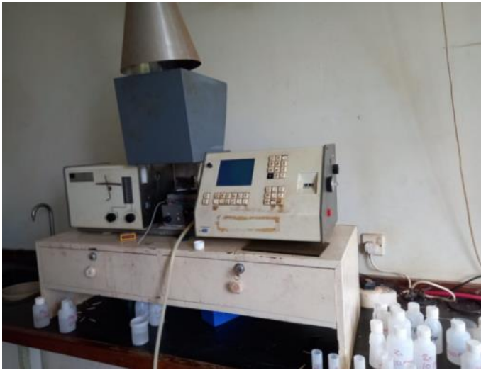
Figure 3: Atomic Absorption Spectrometry instrument used for analysis.
