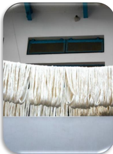
Fig. 3.3b Drying of Silk Hanks after Degumming
