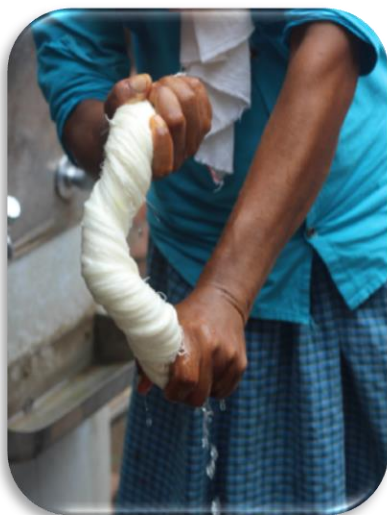
Fig. 3.3a Degumming of Silk Hank
