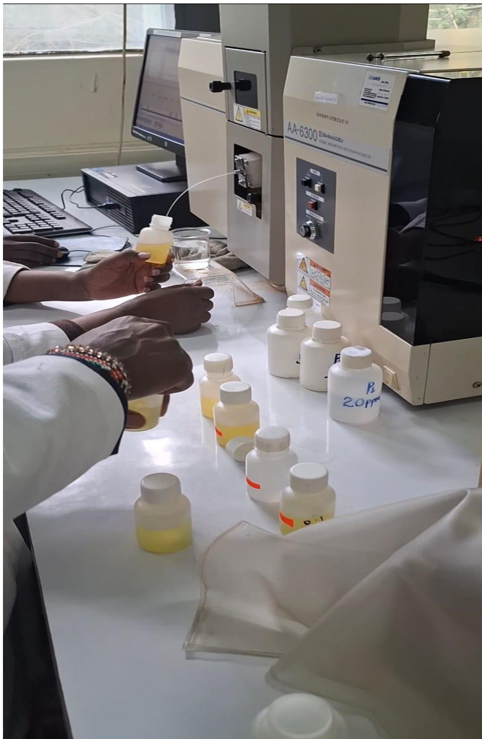
Figure 2 A photo showing analysis for heavy metals using AAS
