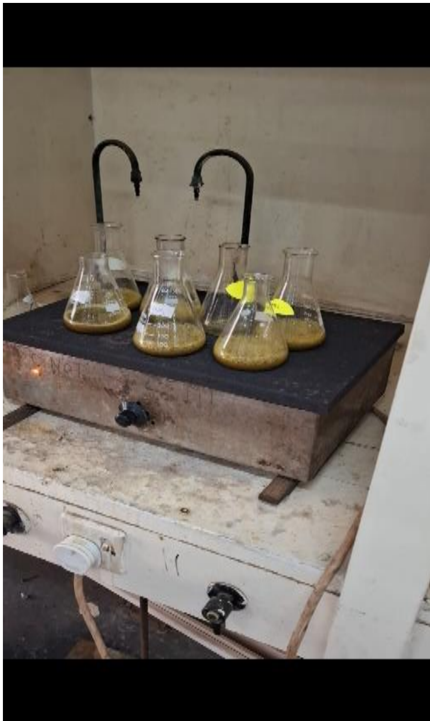
Figure 1 A photo showing digestion of the soil samples
