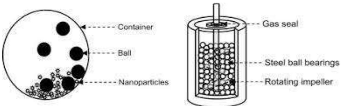
Figure 7 – High energy ball milling technique [24]
