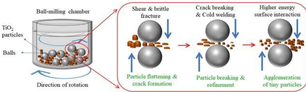
Figure 5 – High energy ball milling [27]
