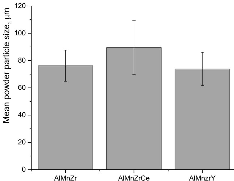
Figure 15 – Powder particle size for the alloys studied
