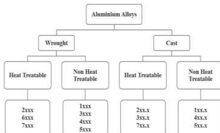
Figure 1 – Classification of aluminum alloys [7]
