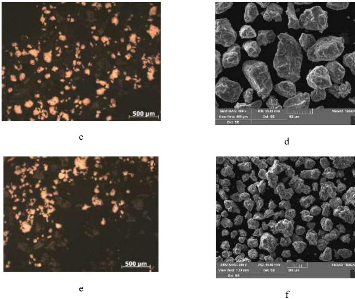
Figure 14 – Granular morphology of of (a) Al-Mn-Zr from TEM (b) Al-Mn-Zr from SEM (c) Al-Mn-Zr-Y from TEM (d) Al-Mn-Zr-Y from SEM (e) Al-Mn-Zr-Ce from TEM and (f) Al-Mn-Zr-Ce
