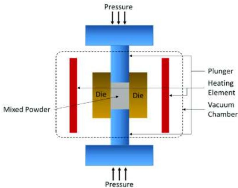
Figure 11 – Schematic setup for hot press sintering [49]
