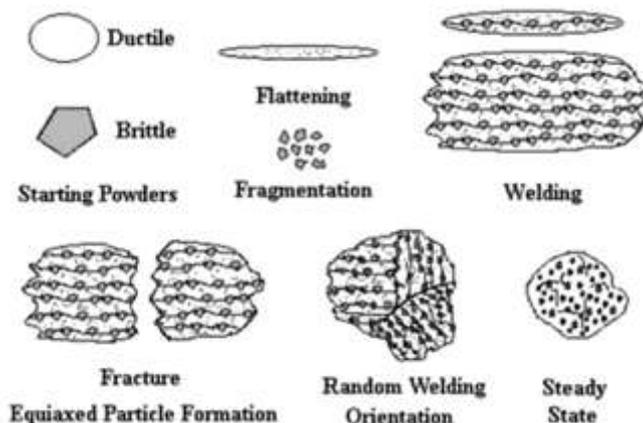
Figure 11 –. The different stages of mechanical alloying in ductile-brittle system [46]
