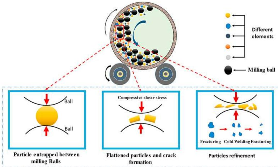
Figure 4 – Overview of mechanical alloying [25]
