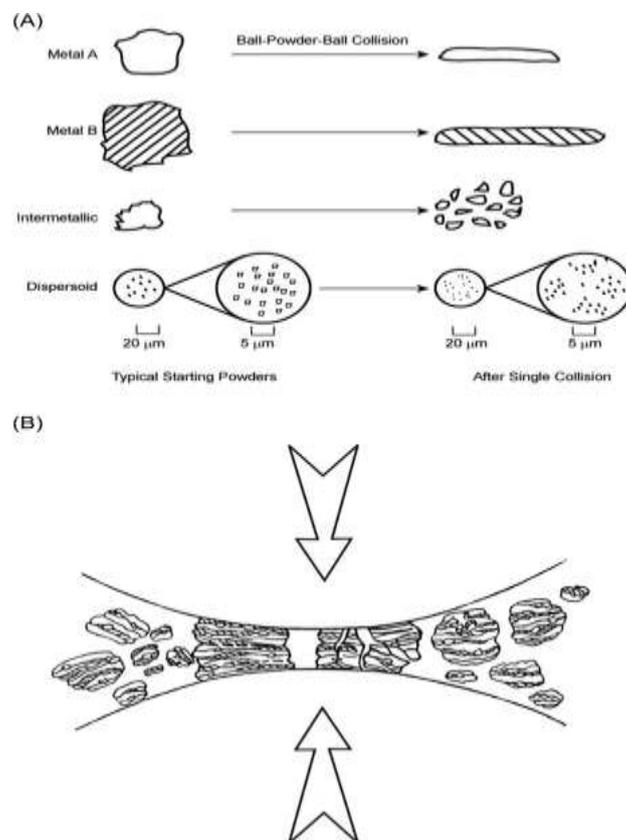
Figure 9 – Events that occur during the ball-to-powder impact [25]
