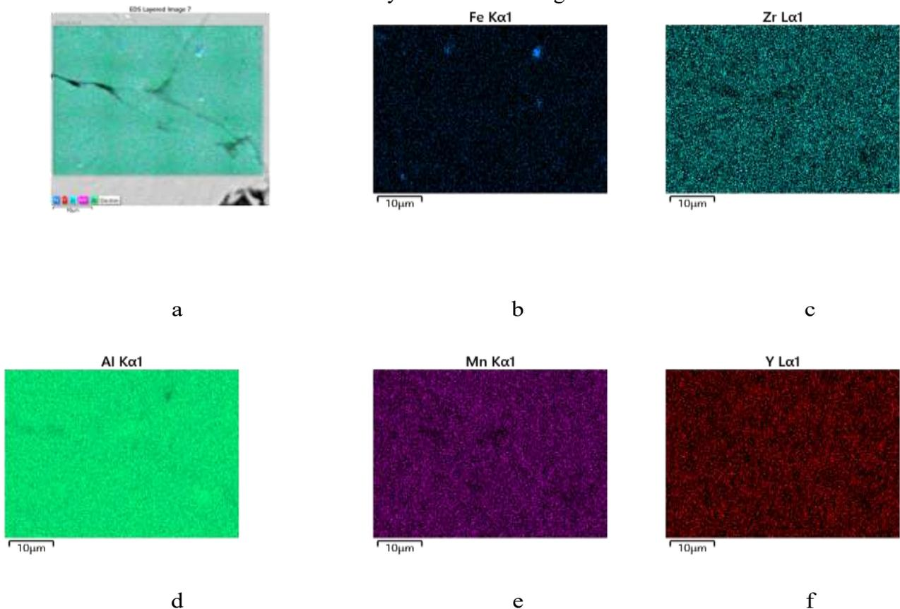
Figure 21 – Elemental distribution in 350 and 450 HPS alloys (a)EDS Image (b) Fe; (c) Zr (d) Al (e) Mn (f)
