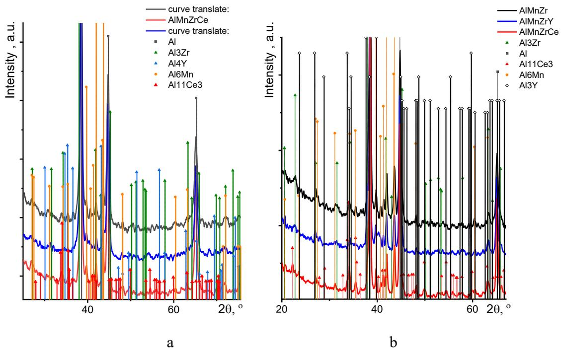
Figure 18 –XRD representation of alloys compacted at 350 °C (a) and 450 °C (b)
