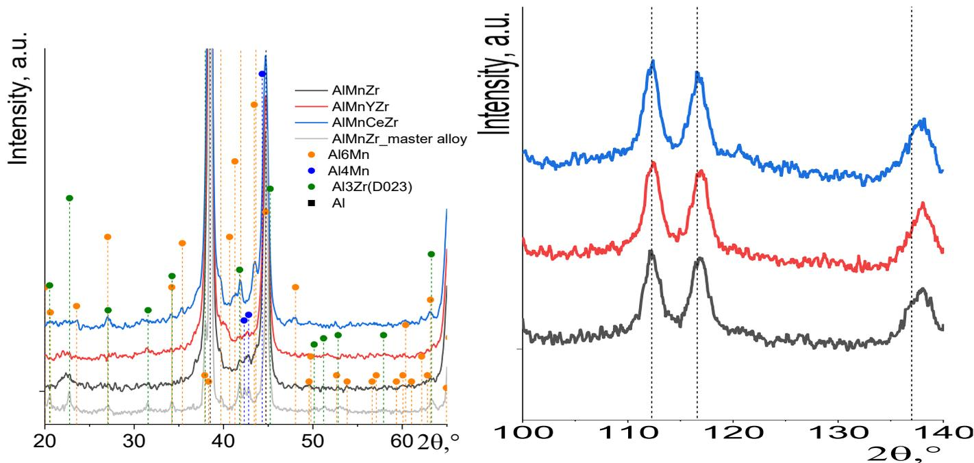
Figure 16 – XRD representation of alloys milled alloys
