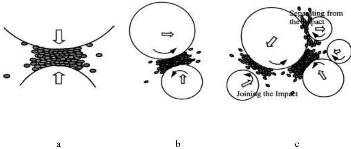
Figure 6 – Mechanisms of mechanical alloying (a) head on impact (b) joining the impact (c) multi ball impact [30]
