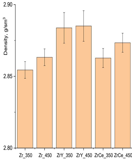
Figure 17 – Density values for the alloys after sintering at 350 and 450 °C
