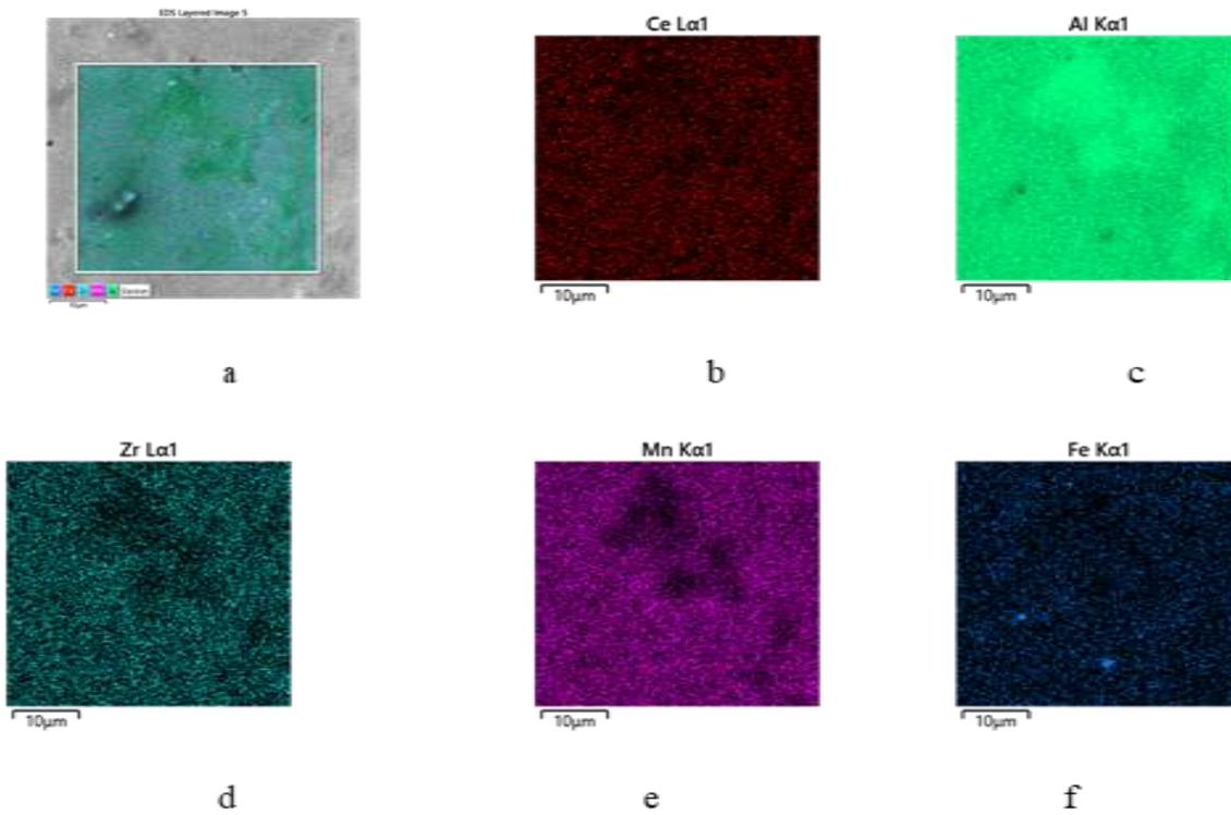
450HPS Compact (After 4 Hours of Annealing) Annealing increased observable coarsening and the creation of intermetallic-rich zones, as illustrated in figure 21 below especially in Mn and Ce areas. Despite the increased particle size, the elemental distribution remained relatively uniform. This result is consistent with the findings of [16] [15] who found that RE additions impacted grain boundary stability and increased heat resistance.
