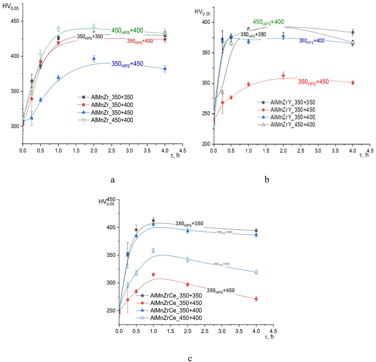
Figure 19 – Micro hardness values at different temperature of (a) Al-Mn-Zr b) Al-Mn-Zr-Y and (c) Al-Mn-Zr-Ce
