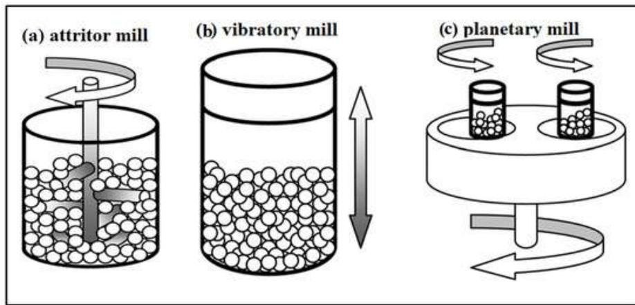
Figure 8 – Types of ball milling [31]
