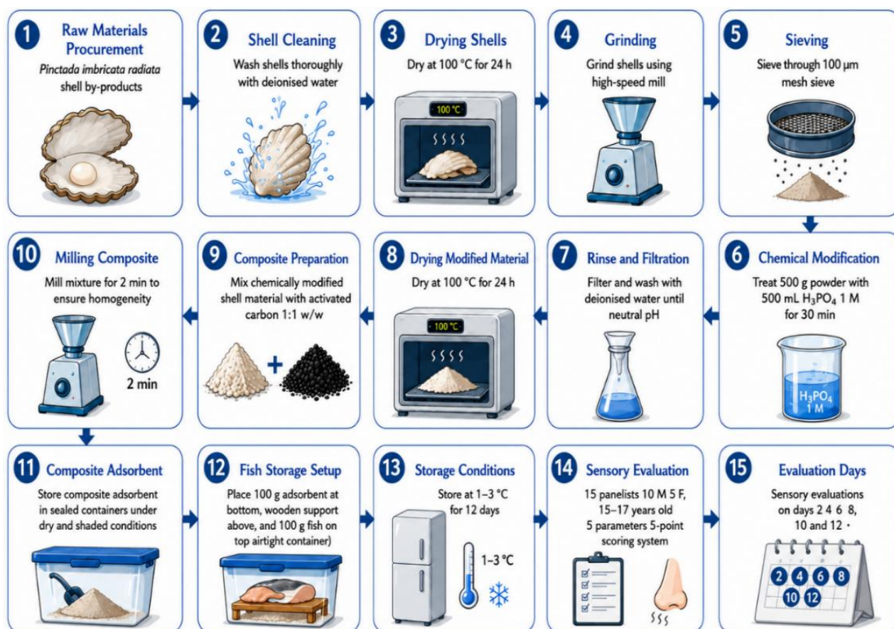
Fig. 1. Schematic representation of Pinctada imbricata radiata shell waste processing and preparation of the composite material for odour-control applications.
