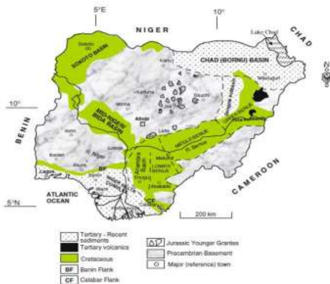
Fig. 1. Geological map of Nigeria showing the major geological Components, Basement, Younger Granites, and Sedimentary Basins [23].
