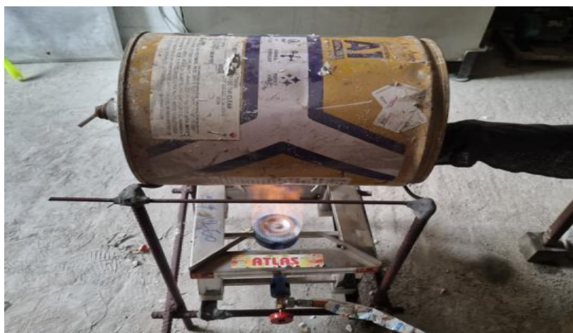
Figure 2: Configuration of the laboratory-scale pyrolysis reactor, heated by an external gas burner.
