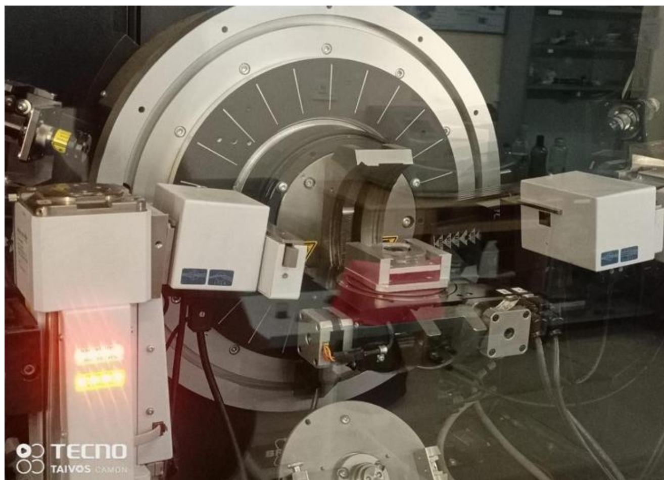
Figure 5: X-ray diffraction instrument used for structural analysis of the synthesized carbon material.
