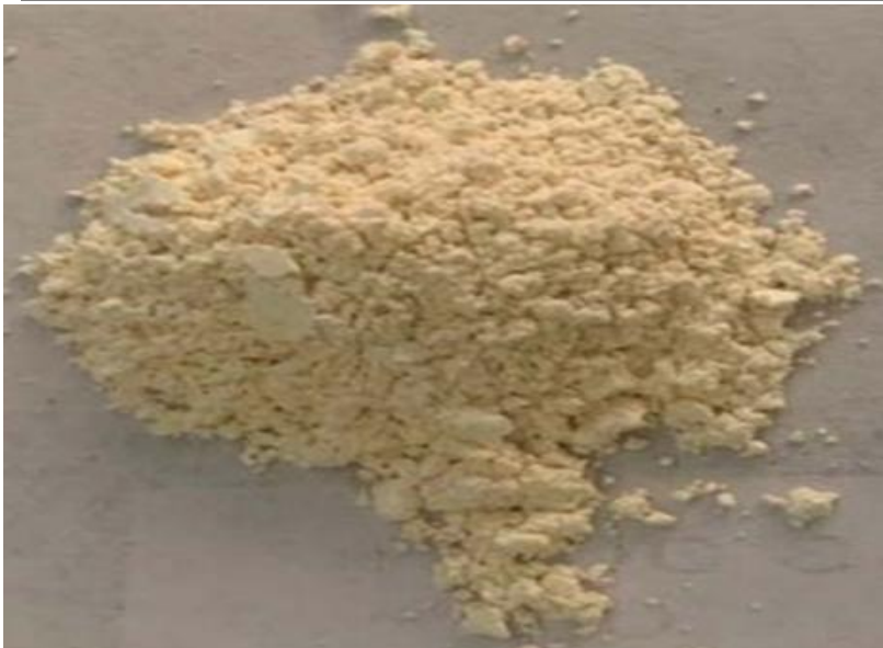
Figure 1: Zeolite crystallized at 105°C with a particle size of 60-80nm
