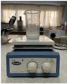
Fig.10. Zeolite, ZnO and Pectin dissolved in deionized water stirred on a hot plate.
