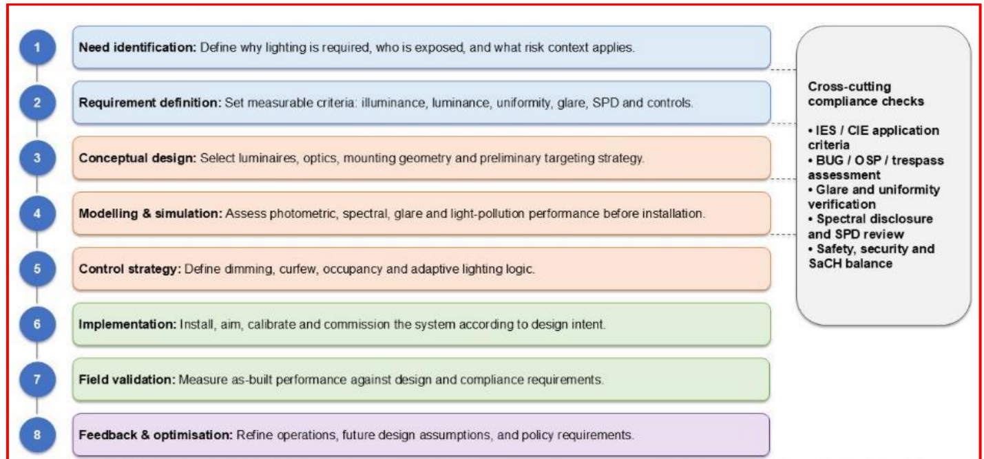
Figure 2. Performance-Based Outdoor Lighting Design Workflow
