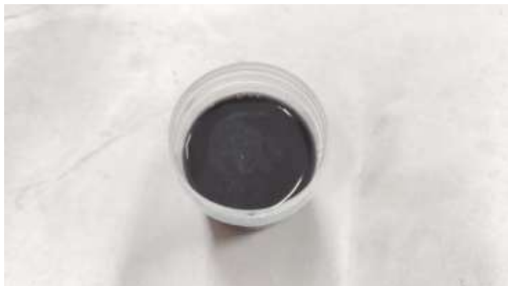
Figure 2. Photograph of the eco-friendly carbon-based ink prepared from plastic pyrolysis-derived carbon and recycled tea leaf extract. The formulation exhibits a homogeneous deep black appearance without visible phase
