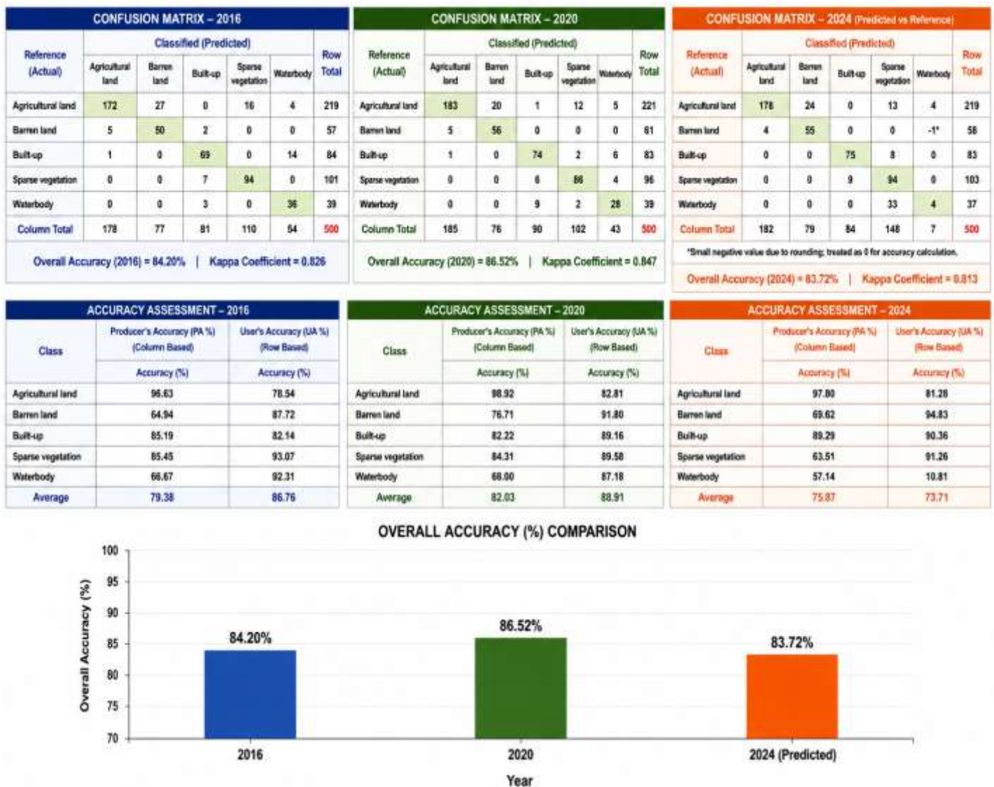
Figure 14: Comparative accuracy assessment of LULC classification and CA-ANN prediction for 2016, 2020, and 2024, showing confusion matrices, producer's accuracy, user's accuracy, and overall accuracy.
