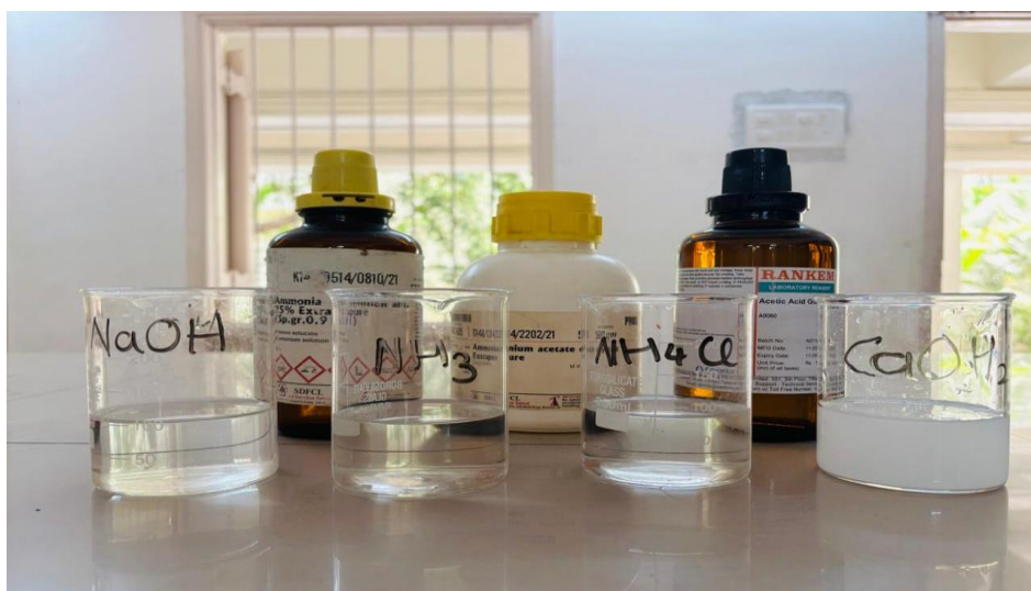
Figure 2: Prepared solutions of NaOH, NH 3 , NH 4 Cl, and Ca(OH) 2 with the corresponding analytical-grade reagents
