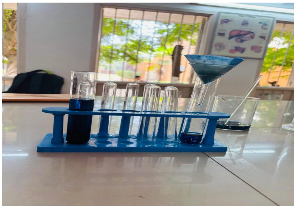
Figure 1: Filtration of the hydroethanolic Clitoria ternatea flower extract through filter paper to obtain a clear pigment solution
