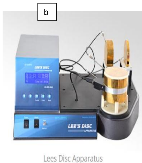
Figure 4: Devices are used to evaluate the specimens: a – mechanical properties measuring device (Tensile); b – Hilmarc's Lee's Disc apparatus for thermal conductivity measurement
