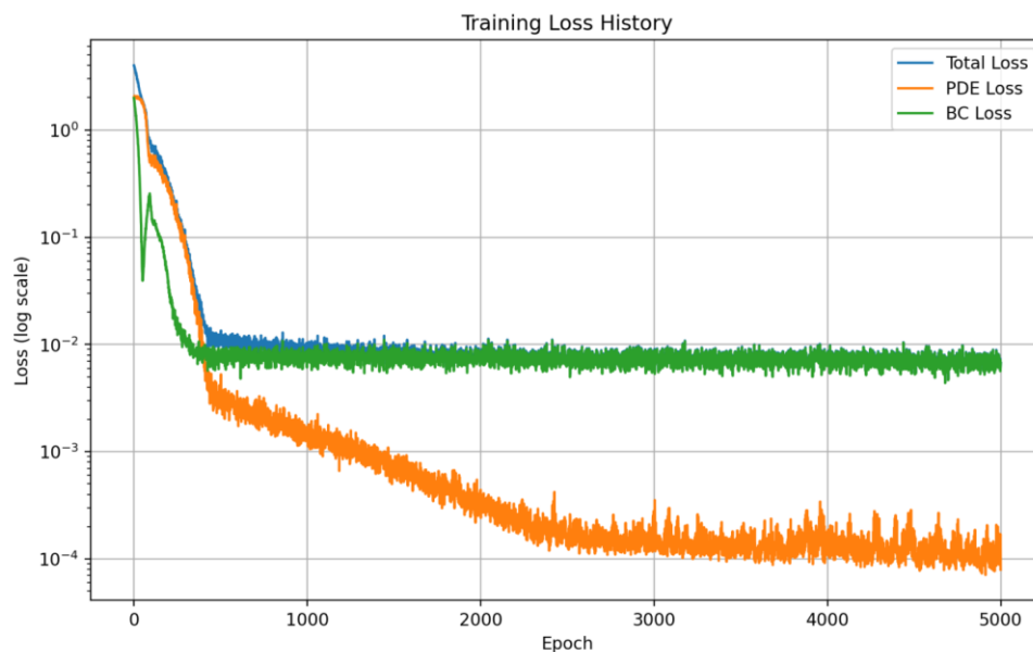
Fig 12 Training Loss history for the solution of MA PDE as well as boundary condition loss.
