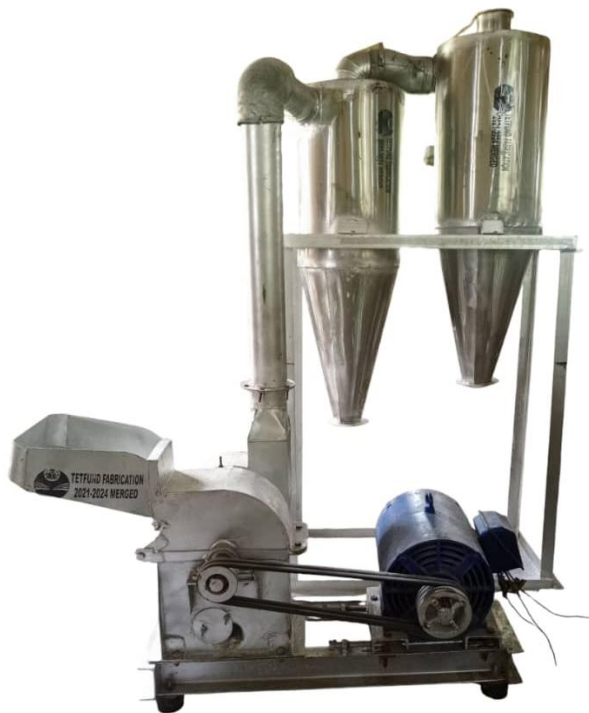
Plate 1: The fabricated Hammer Mill
