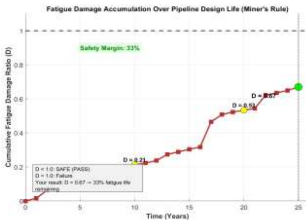
Figure 7. Cumulative fatigue damage accumulation over the 25-year pipeline design life.
