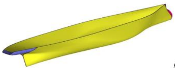
Figure 1. Three-dimensional geometry of the S-175 containership.
