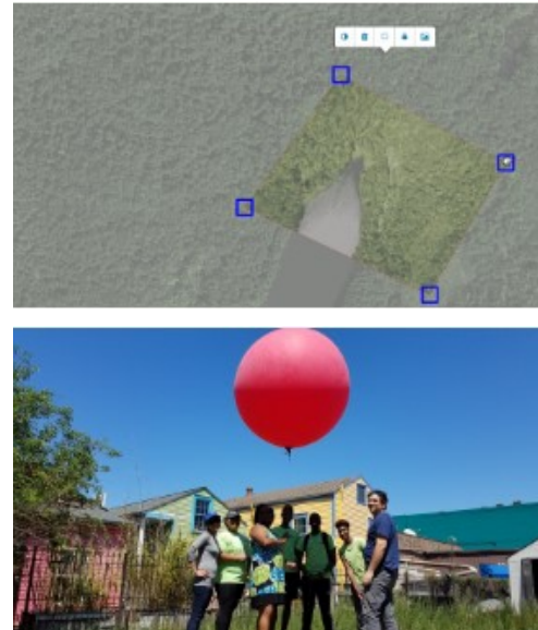
Fig5: Capturing earth photos through balloon & map construction from image
