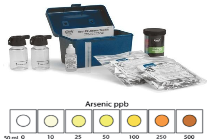
Figure 2: HACH EZ Arsenic Test Kit and Colour Chart
