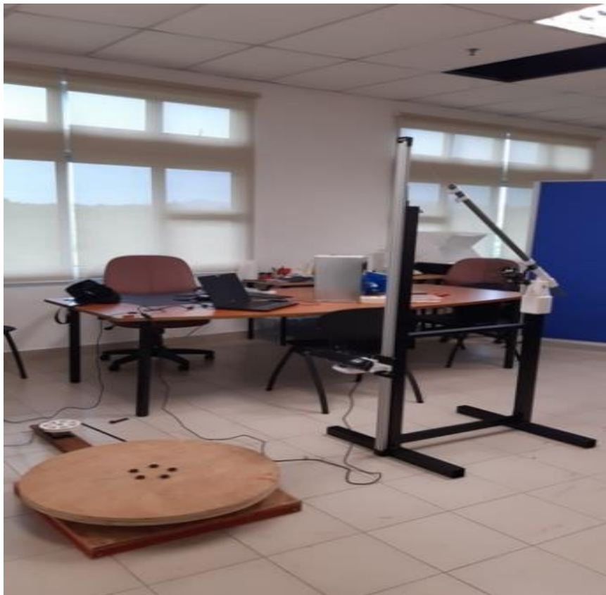
Fig. 2: The low-cost 3D scanning which has Kinect stands and a turntable platform (Source, Muhammad Sukor Romat, 2024).
