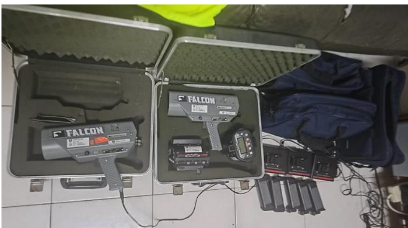
Figure 1: Radar Gun & Laser Gun for the Spot Speed Study at Meru Tunnel
