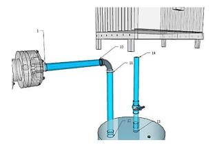
Link a <sup>3</sup>/<sub>4</sub>-inch pipe (15) to an additional water storage unit. This pipe should connect to a <sup>3</sup>/<sub>4</sub>-inch 45°-degree elbow. Extend this assembly by adding another <sup>3</sup>/<sub>4</sub>-inch pipe and securing it with a <sup>3</sup>/<sub>4</sub>-inch ball valve. Finally, connect this pipe to the water filtration device.
