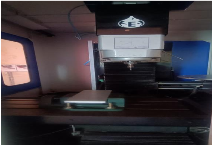
Figure 2: CNC Machine Bed and Tool setup (Flat End Mill cutter)
