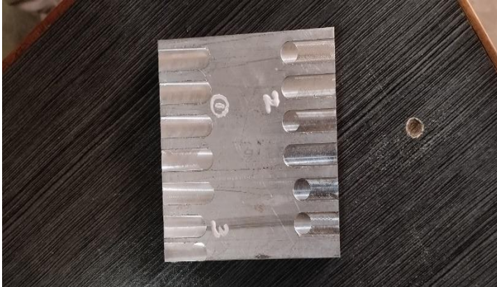
Fig 4: Aluminum plate after Flat cutting using CNC
