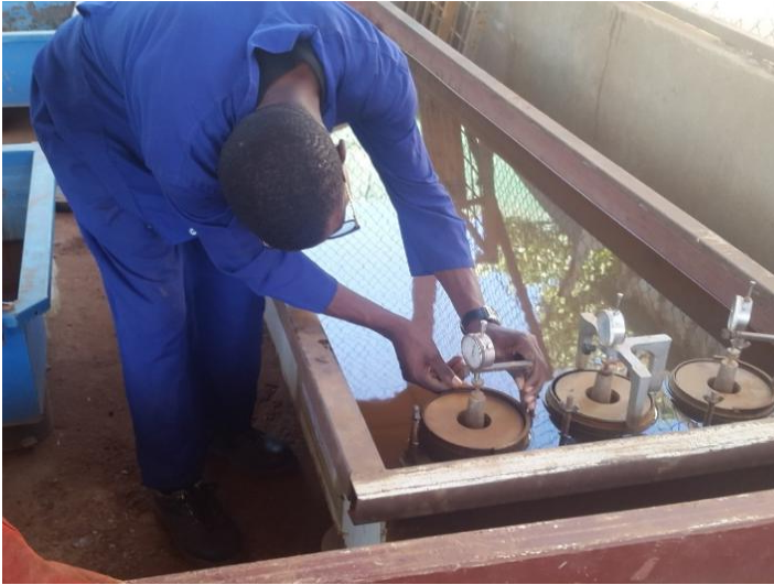
Figure 2: Soaking of CBR specimens
