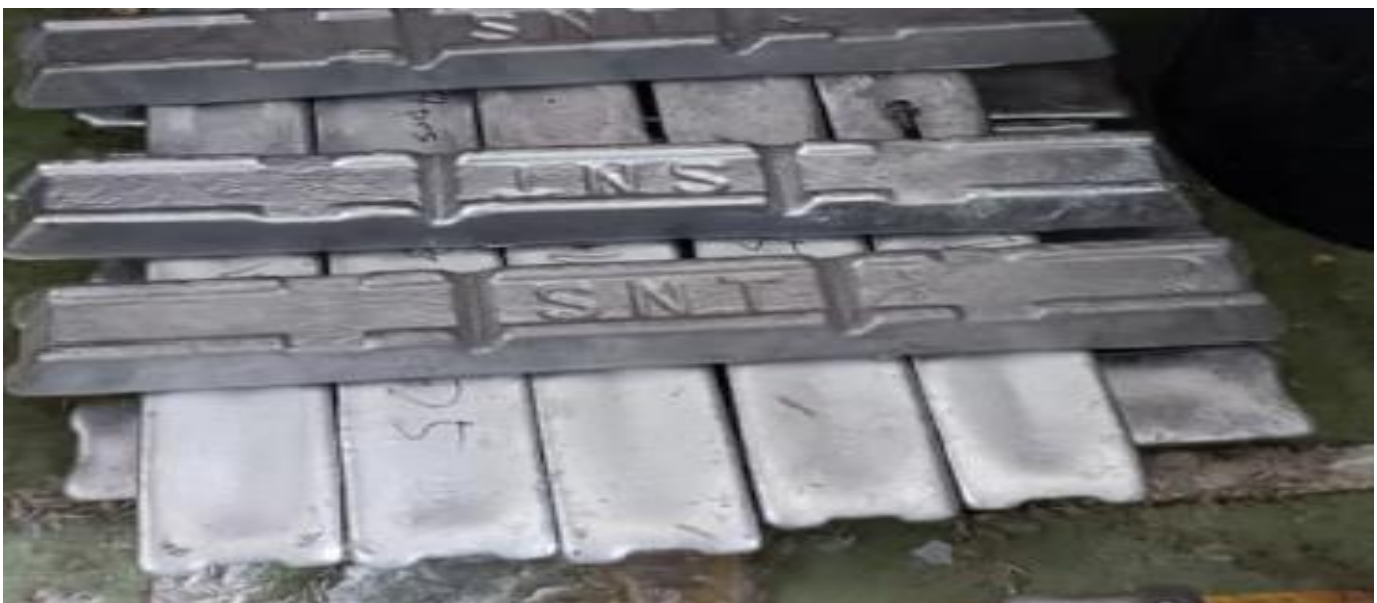
Figure 2.1.2: Aluminum Ingot (A356)
