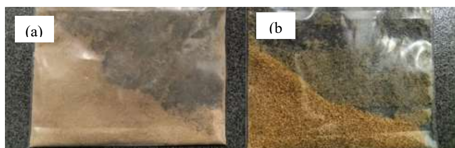
Figure 3: Image of SDW fiber (a) before alkaline treatment and (b) after alkaline treatment
