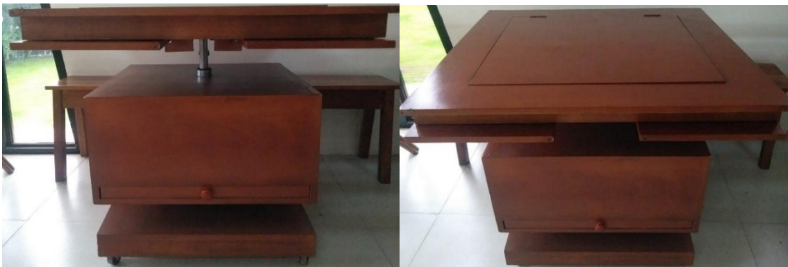
Figure 12: Actual photo of the ergonomic garment table with hydraulic height adjustment mechanism
