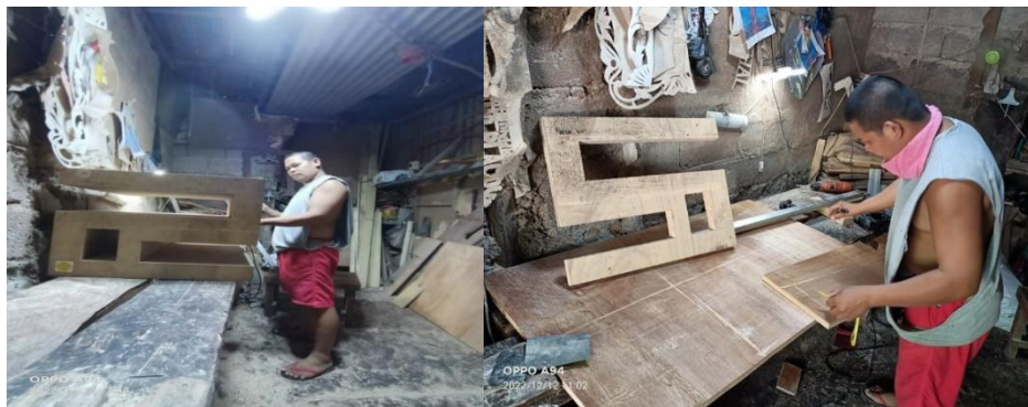
Step 3. Lay outing the wood by measuring and marking its final measurements
