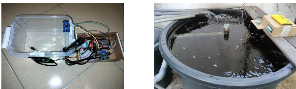
Fig. 3 Testing the prototype of aquaponic monitoring system
