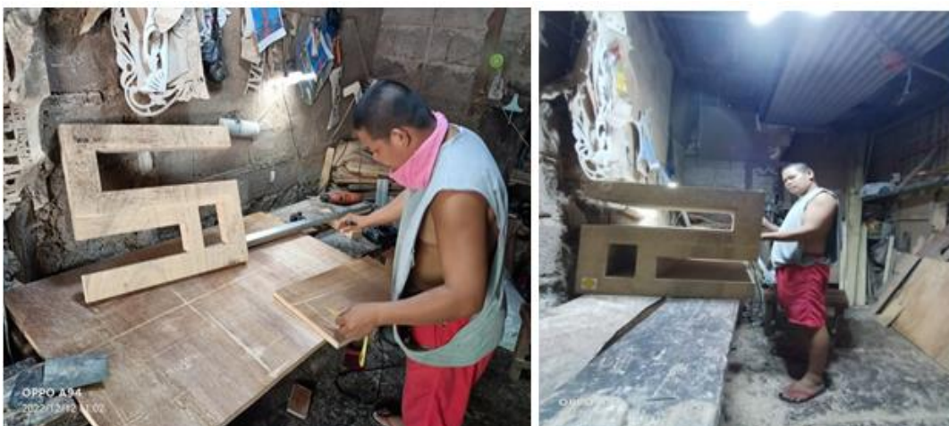
Step 3. Lay out the wood by measuring and marking its final measurements
