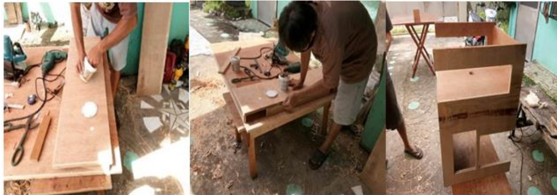
Step 5. Assembling the pieces of wood using adhesives and fasteners.
