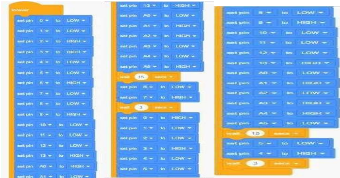
Figure 4. Traffic Light System Tinkercad Blocks
