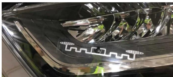
Fig 1 A RFID Sticker placed at headlights for toll payment in Malaysia
