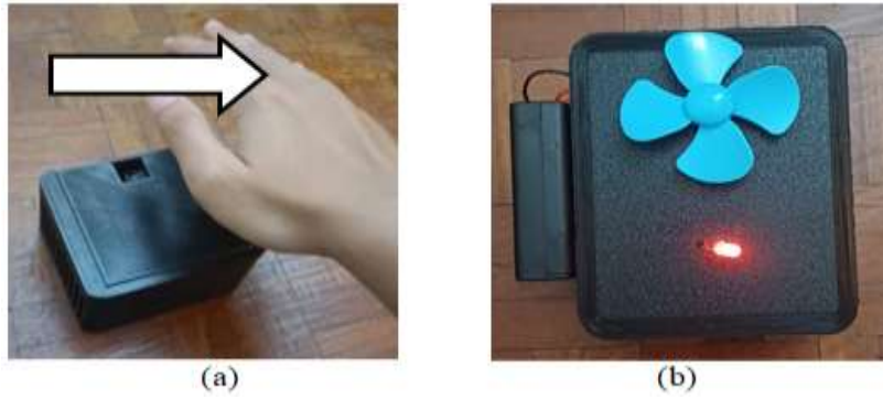
Figure 12: Lamp Control Using Right Wave Gesture: (a) Right Wave Gesture, and (b) LED ON
