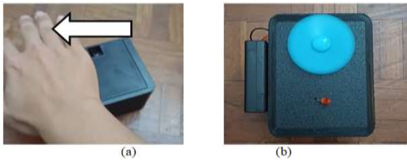
Figure 13: Lamp Control Using Left Wave Gesture: (a) Left Wave Gesture, and (b) LED OFF
