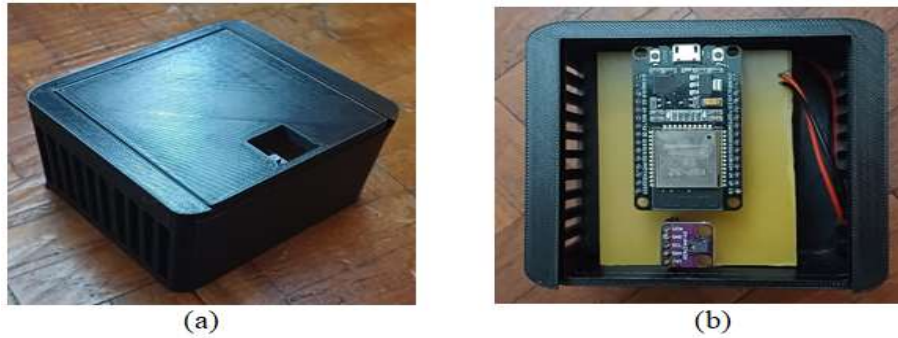
Figure 9: Transmitter Prototype Views: (a) Overall View, and (b) Internal View
