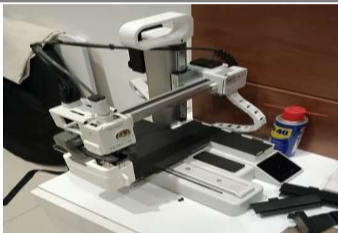
Figure 6: Bambu A1 Mini 3D Printer Used for Prototype Fabrication
