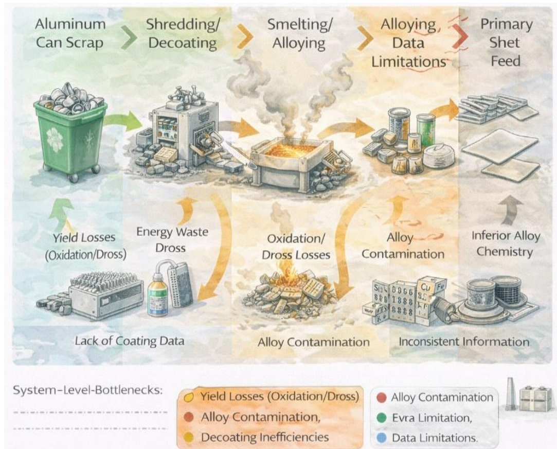
Figure 18. System-level bottleneck map for aluminum can recycling, highlighting yield losses (oxidation/dross), alloy contamination, decoating inefficiencies, and data limitations. Adapted from Padamata et al. (2021); Steglich et al. (2020); Van den Eynde et al. (2022).
