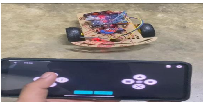
Figure 1 The robot car being controlled by smartphone using Bluetooth connection.
