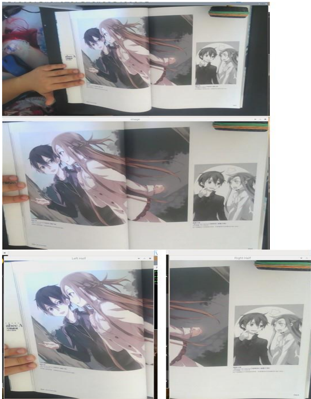
Figure 6: (a) Original image. (b) Result of image cropping. (c) Result of left page. (d) Result of right page.
