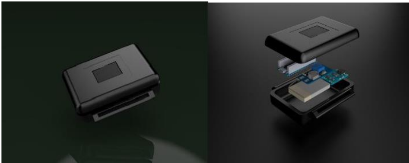
Figure 2.1 3D View of the Bracelet Enclosure Design
